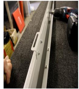
Attach 3 x silver cross bracing to each side using M5 nuts supplied.
